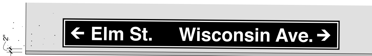
CONCRETE BEAM MOUNTED SIGNS ALIGN WITH BOTTOM OF BEAM
