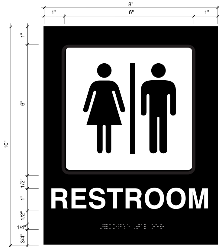
CO3 - RESTROOM PLAQUE - TYPICAL SCALE: 3/8"=1"
