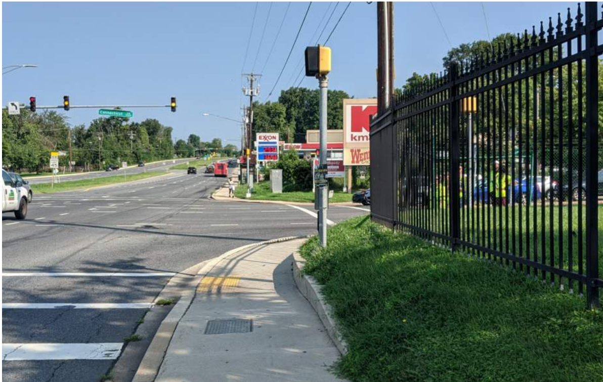
Photo 6.15. Sight line of crossing obstructed by fence line along NB MD 97 approach.
