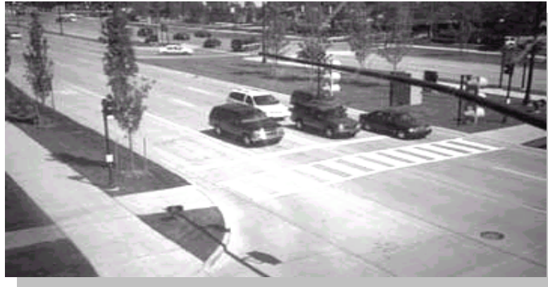
The “ladder” pattern is more visible to motorists and requires less maintenance if painted to allow the tires of motor vehicles to track between the paint lines. (Photo by Peter Lagerwey)
