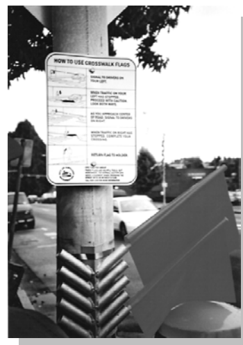
A crosswalk equipped with bright red flags that pedestrians can carry while crossing the street to alert motorists to their presence.
