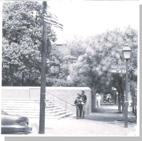
A pedestrian “walk / don’t walk” signal with a countdown timer to let pedestrians see numerically much time they have to cross the street.
