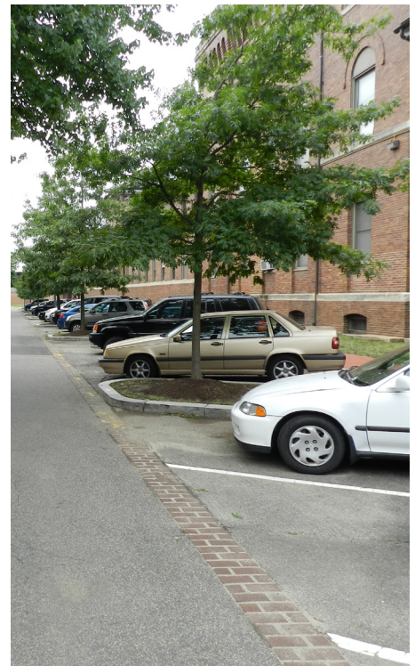
Figure 4-6. Back in angle parking (City of Kelowna, BC, Canada)
