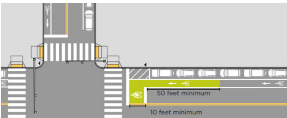
Figure 6-21. Bike box detail from Montgomery County Bicycle Master Plan Appendix B: Facility Toolkit
