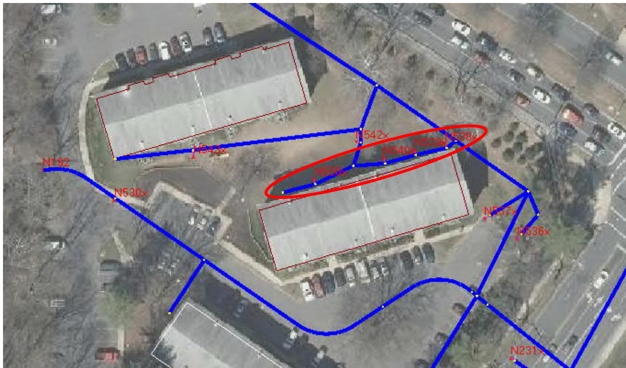
Figure 143 - Map of ICPR 2D model showing inlet locations with labeled node numbers
