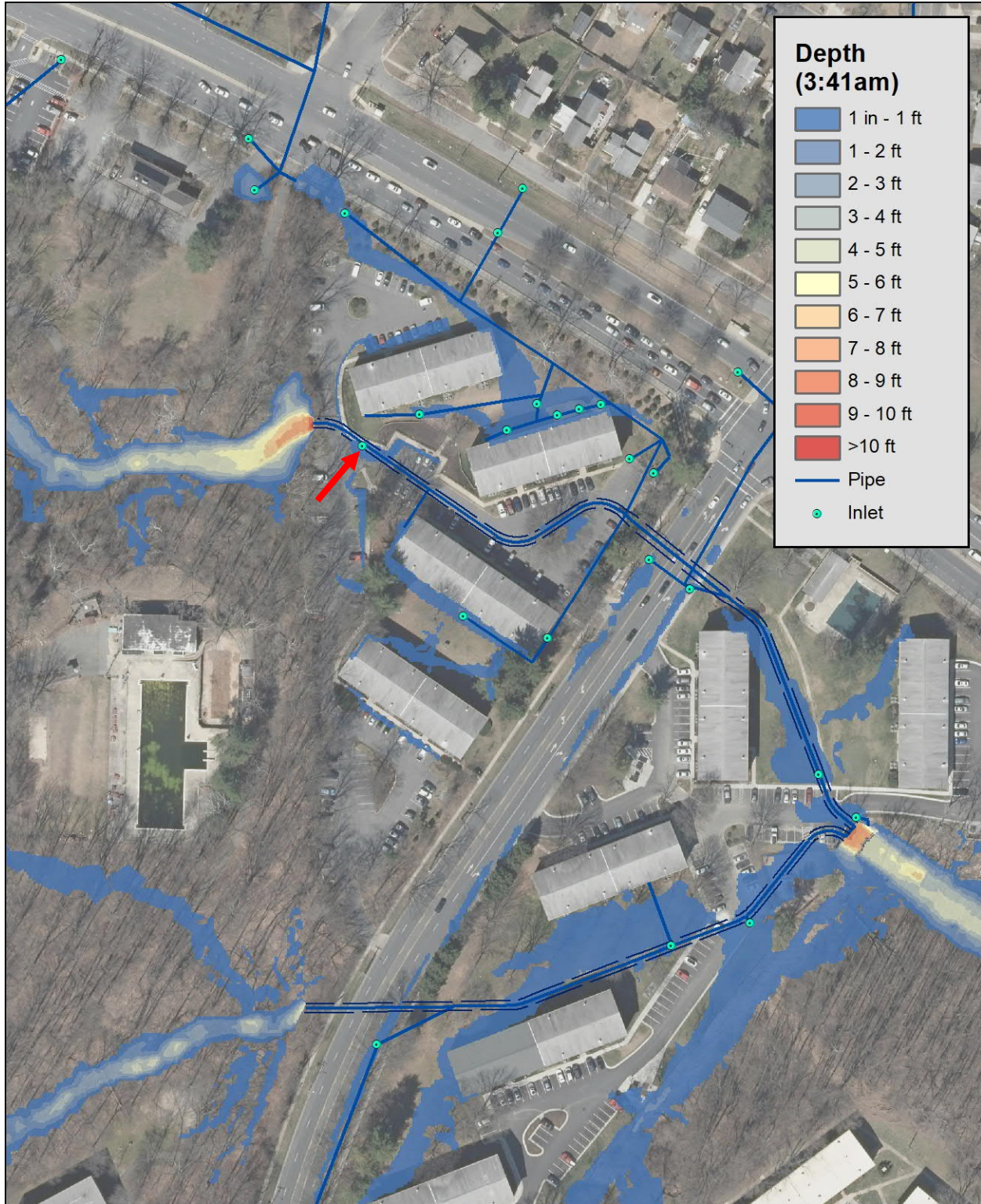
Figure 134 - 2D Simulation Depth Map, 3:41 am Stormwater has started to surcharge out of the first inlet from the upstream end that is in the top slab of the culvert.
