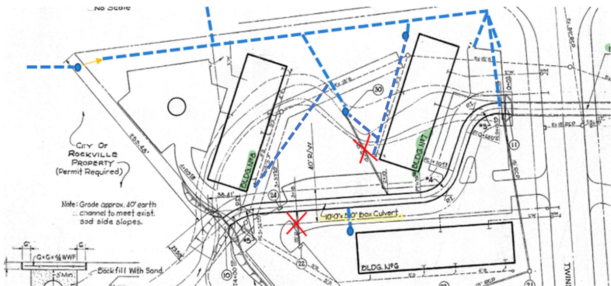
Figure 64 - Excerpt of 1966 Permit Plans showing inlets (blue circles), storm drain pipes (blue dashed lines), concrete flume (yellow arrow) and pipes that do not match the actual surveyed conditions (red X's).
