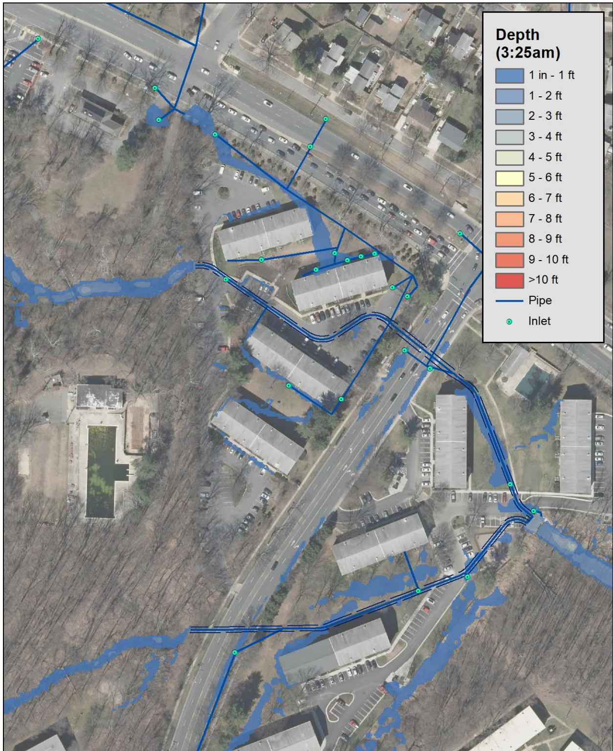
Figure 133 - 2D Simulation Depth Map, 3:25 am Stormwater that has overwhelmed the open channel at the Northwest Corner of the Rock Creek Woods Apartments Property has reached the low point between Buildings 7 and 8.
