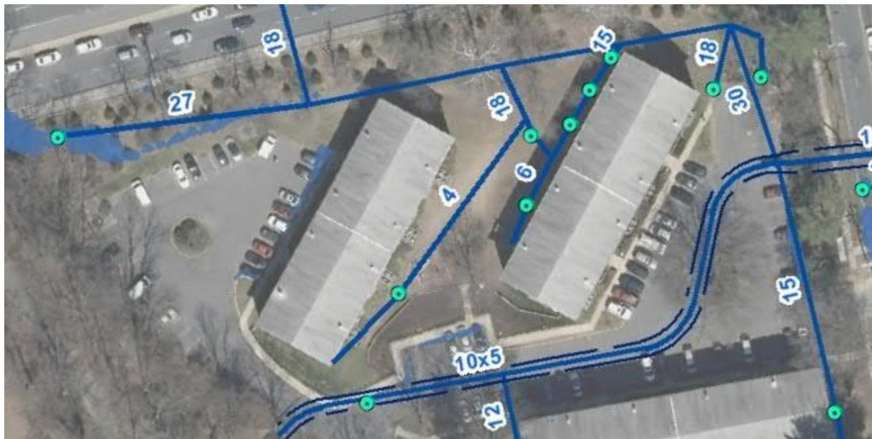
Figure 66 - Existing Storm Drain System with Pipe Diameters (inches) and Culvert (Dashed line, dimensions in feet).
