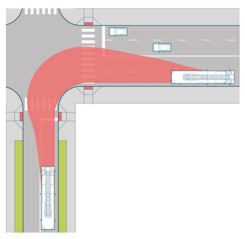
Figure 6-9: Graphic of allowable control vehicle encroachment at intersection
