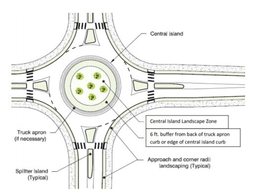
Figure 6-17. Typical roundabout design elements (Source: Maryland State Highway Administration, Roundabout Design Guidelines, 2012)
