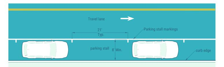
Figure 5-5. Illustration of a typical on-street parallel parking space with dimensions
