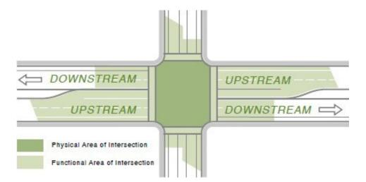
Figure 6-2: Functional and physical areas of an intersection (Source: FHWA Access Managemet in the Vicinity of Intersections)
