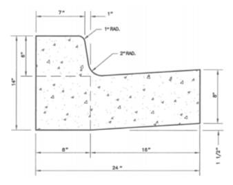
Figure 5-15. Montgomery County curb and gutter dimensions
