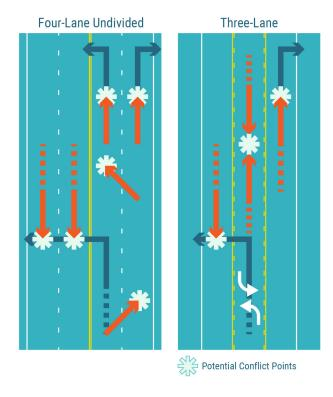
Figure 9-4: Example of the reduced number of conflict points on a 4-lane to 3-lane roadway conversion (Source: Federal Highway Administration, Adapted from Welch, T. The Conversion of Four Lane Undivided Urban Roadways to Three Lane Facilities. 1999.)
