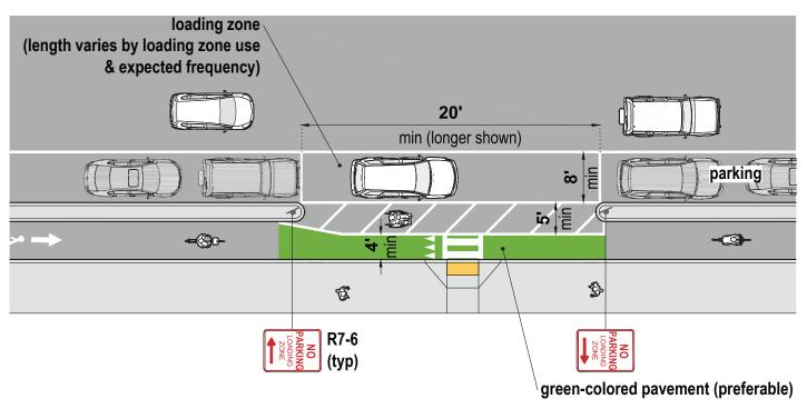
Figure 5-13. Example guidance for passenger loading zone with a separated bike lane
