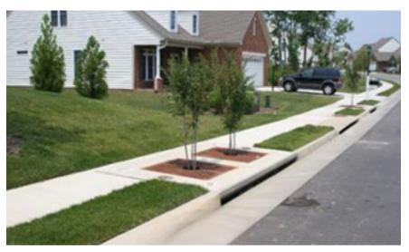
Figure 7-8: Examples of other green infrastructure BMPs (Source: Montgomery County Department of Environmental Protection)
