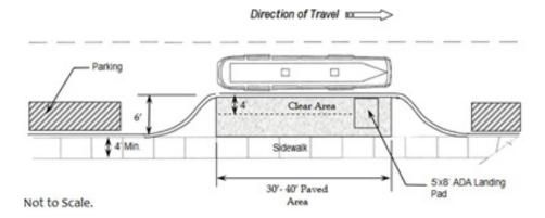
Figure 6-24. Bus Bulb design (Source: WMATA's Guidelines for the Design and Placement of Transit Stops)
