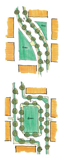
Figure 9-10. Alternative options for roadway geometry in suburban contexts
