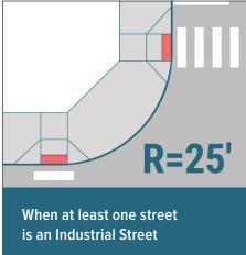
Figure 6-5: Corner radius design guidance
