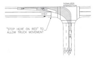
Figure 6-10. Recessed stop bar
