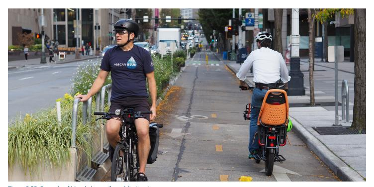
Figure 8-23: Example of bicycle lean rails and foot rests
