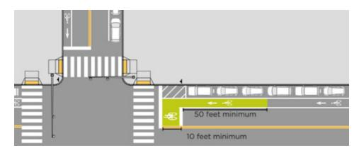
Figure 6-21. Bike box detail from Montgomery County Bicycle Master Plan Appendix B: Facility Toolkit
