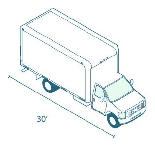
**Montgomery County's** standard design vehicle is a 30-foot single unit truck (SU-30) with a 42-foot turning radius.
