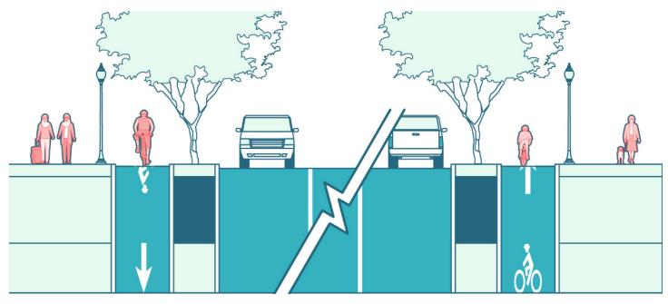
Figure 8-10: One-way Separated Bike Lane, Tree Separated, Permanent Condition: Downtown Street, Town Center Street, Industrial Street
