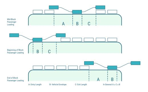
Figure 5-12. Ride hailing pickup/drop-off area diagrams (Graphic content from: ITE Curbside Management Practitioners Guide)
