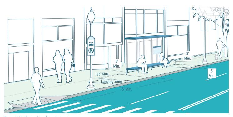
Figure 4-19. Illustration of bus shelter clearances
