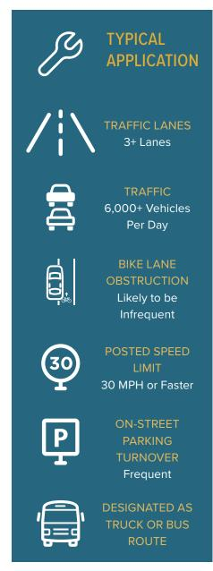
Figure 8-3: Typical application of separated bikeways
