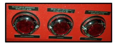
These warning lights indicate if a compartment on the left or right side of the apparatus is left open when the Parking Brake is released (left and right lights), or if the Extend-A-Gun is left raised (center light - Elevation).
