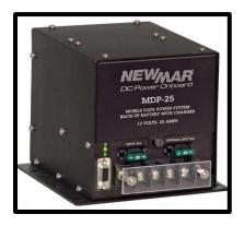
The NewMar MDP-25 mobile data power computer uninterrupted power supply (UPS) with interactive power signals prevents system crashes, and data and hard drive corruption due to low voltage or loss of power. This delay timer switch contains a 9 AH battery that switches on when primary voltage drops, supplying 25 amps of 12V power -- assuring continued operation. An internal 3-step, temperature-compensated charger maintains the MDP-25 reserve battery at full charge.
