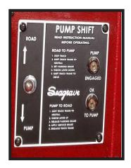
Example of a Pump Shift Panel on the Center Console Control Panel
