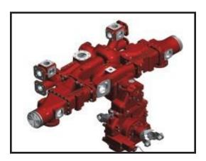
The Waterous fire pump is a two stage (twin impeller) centrifugal water pump. As such, it is classified as a non-positive displacement pump since it does not pump a definite amount of water with each revolution. Rather, it imparts velocity to the water and converts it to pressure within the pump itself.
