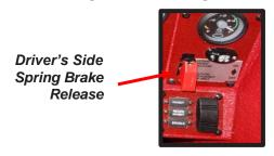
The Spring Brake Release switch is located on the left side of the center control panel.
