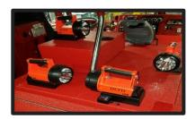
Throughout the cab, these lanterns can be installed. They are set into a Charging Rack that is wired into the electrical system of the apparatus.
