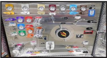
Example of an Upper Section, Pump Panel - Driver's Side
