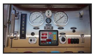
Example of an Upper Section, Pump Panel – Driver's Side
