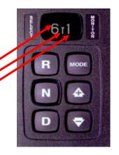
During normal operation when D (drive) is selected, the digital display shows the highest forward range attainable for the shift schedule in use. Abnormal operation is also indicated by the digital display. When all segments of the digital display are illuminated for more than 12 seconds, the ECU did not complete initialization.
