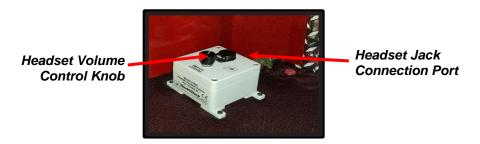
A Remote Headset Station is installed throughout the cab, usually by each occupant's seat,
