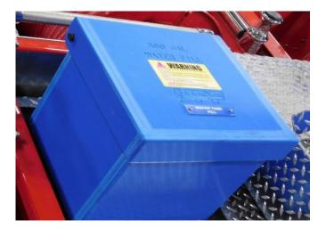
The Water Fill Tower is located on the roof of the pumper, just above and to the right of the Driver's Side Operator Stand. It is a combination vent and manual, water only fill tower with a removable screen and a hinged cover.
