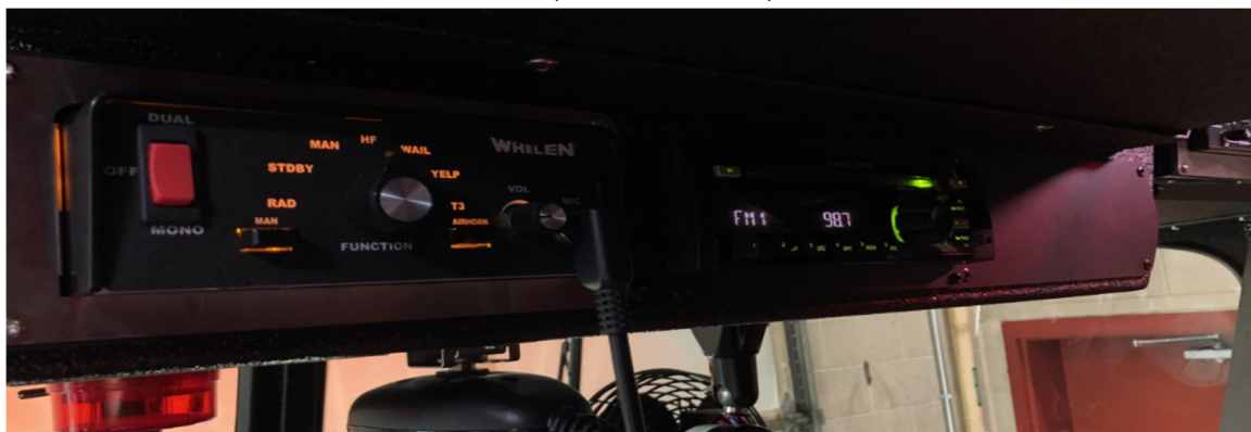
Center Cab overhead- Electronic Siren, AM/FM Radio, Mobile Radio
