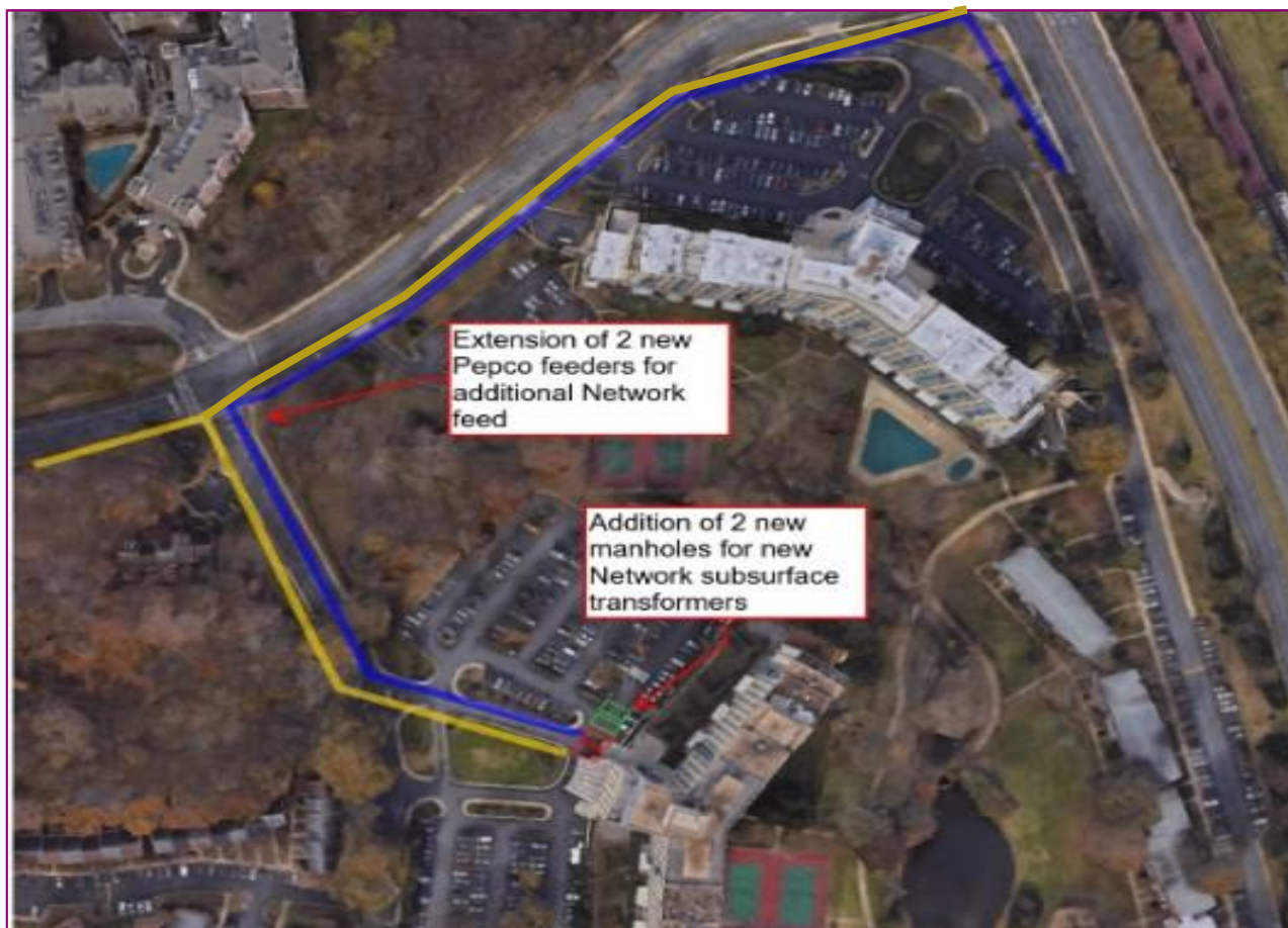
Figure 18 – Concept Drawing – Proposed route of extension of Network Feeder for new load under Option 1
