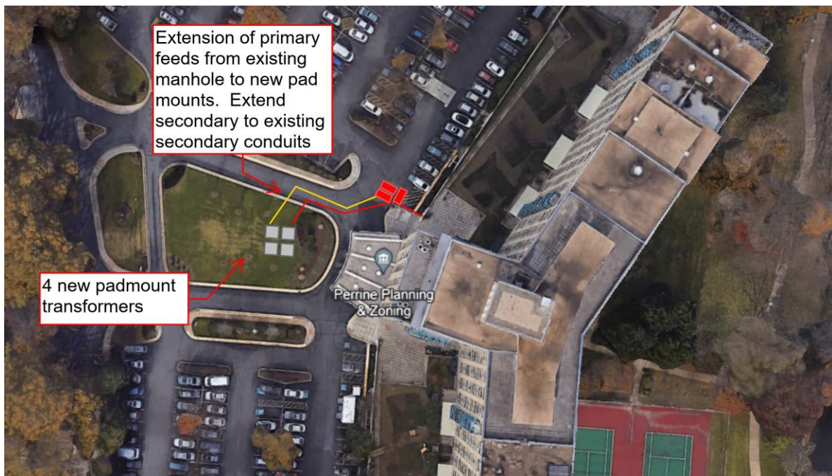
Figure 19 – Concept Drawing – Extension of feeders and installation of radial transformers for future load needs under Option 2
