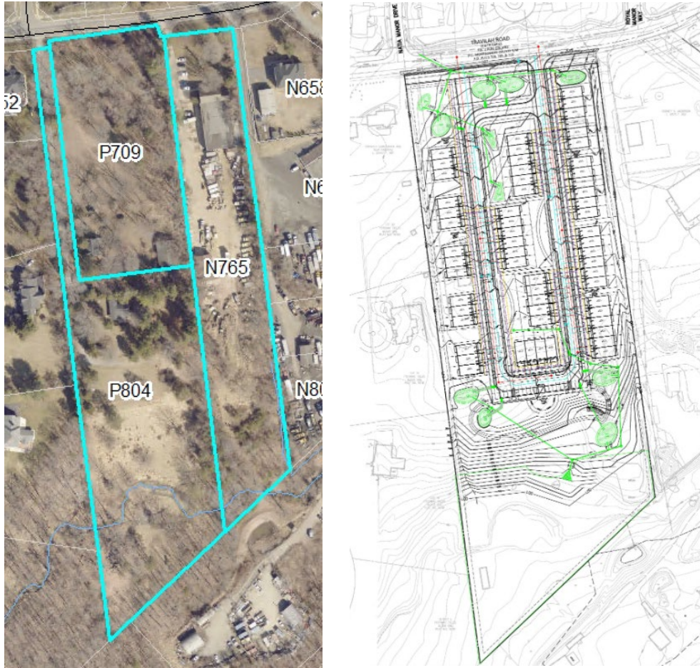
Figure 8. On the left is the parcel layout for the Hurst and Ennis (P804), Blackman (P709), and Johnson (N765) properties; on the right is the utility plan from conditional use application CU202310 showing the proposed townhouse configuration on the combined properties.
