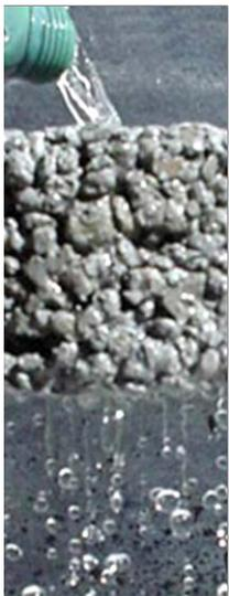
*Water draining through pervious concrete.*
