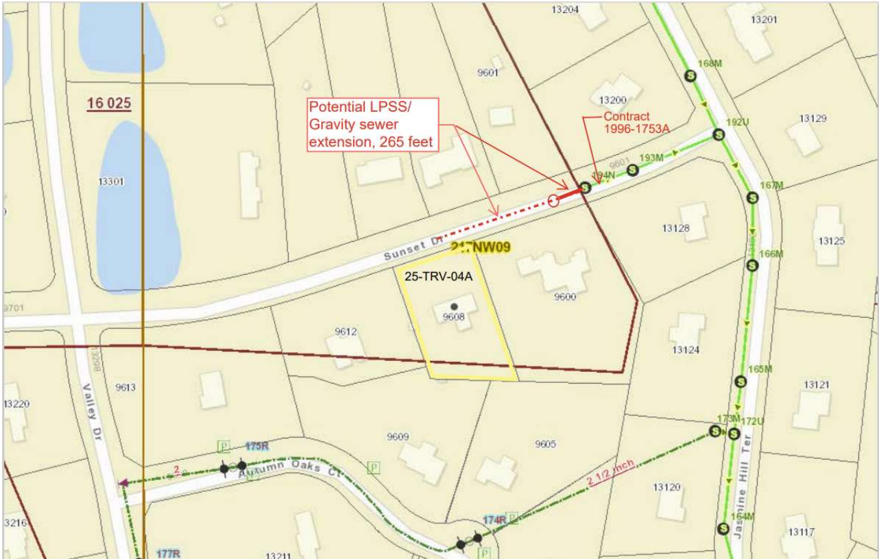
Figure 4: A concept plan for the sewer main extension needed to serve 25-TRV-04A provided by WSSC Water.
