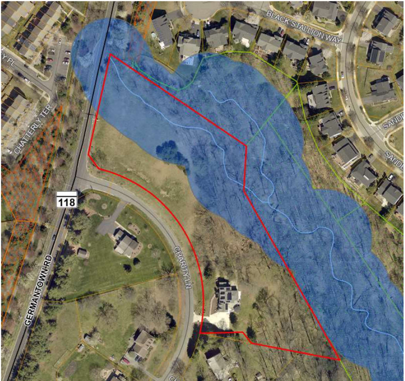
Figure 3: 2023 aerial image of subject property showing approximate extent of a 100-foot stream buffer.
