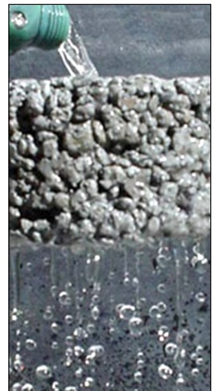
Water draining through pervious concrete.
