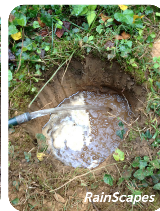
perc test hole, filled
