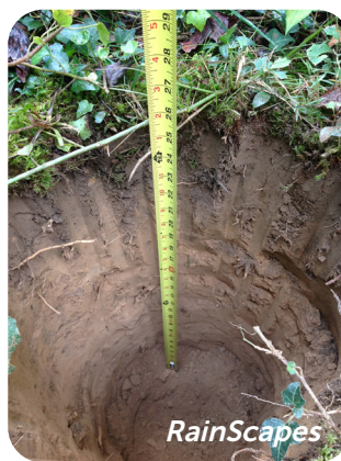
perc test hole, dug
