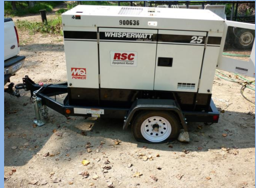
Generator for running pumps
