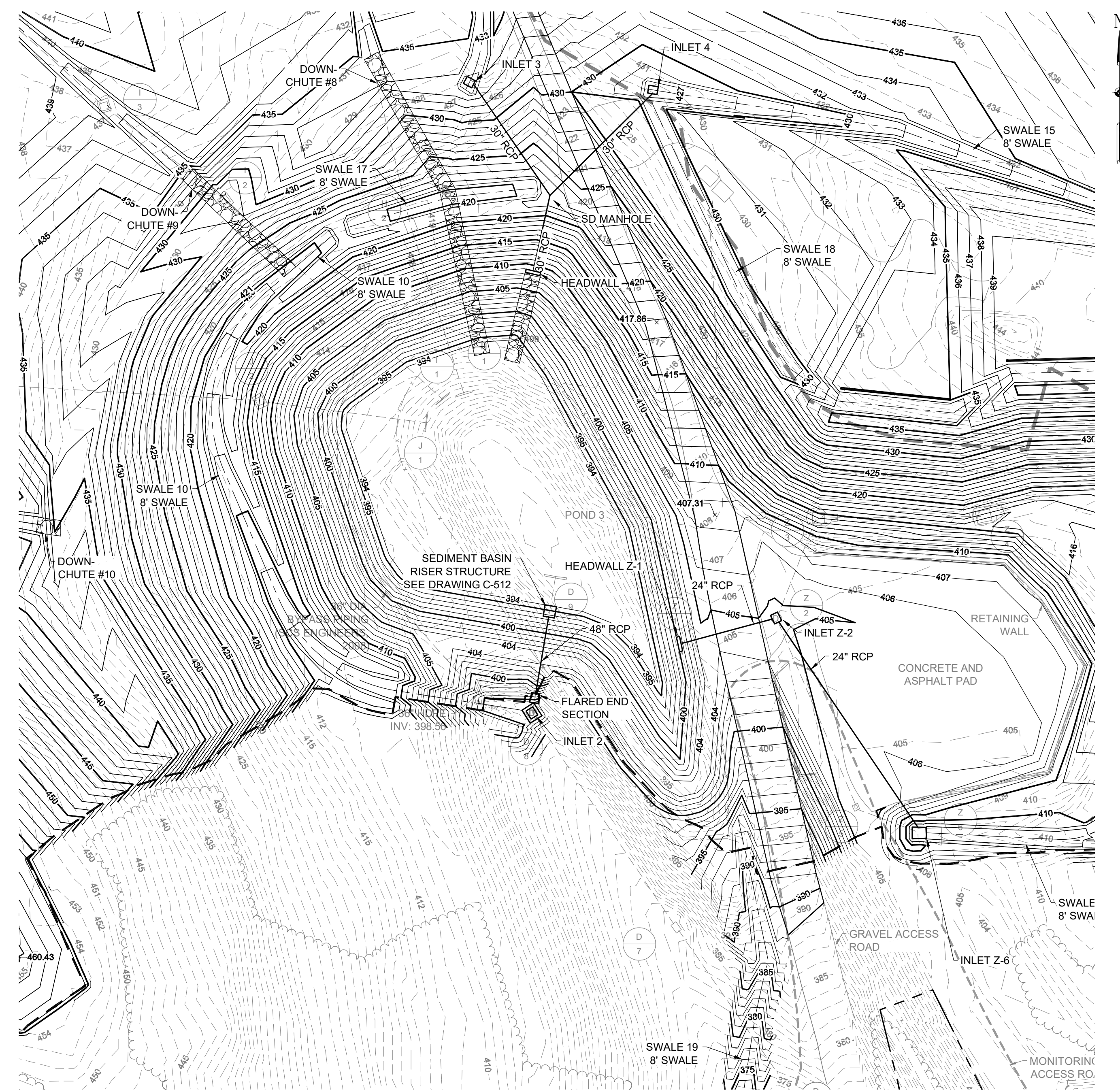
STORM DRAIN PLAN - I-2 TO RISER, HEADWALL TO I-3, AND MANHOLE TO I-4 SCALE: NOT TO SCALE
