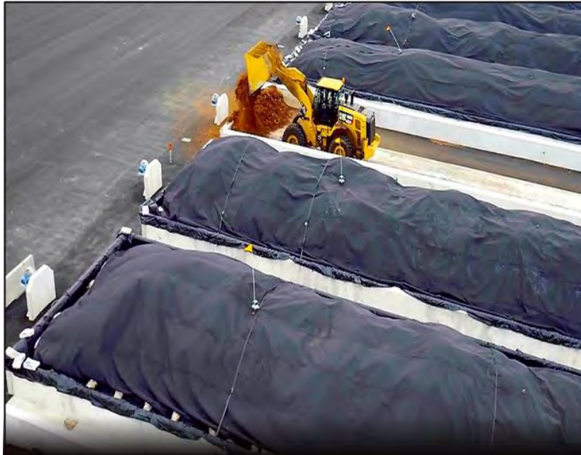
Aerated Static Pile w Membrane at MCYTCF
