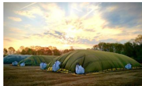
Aerated Static Pile with Microporous Cover (courtesy Prince George's County, MD)
