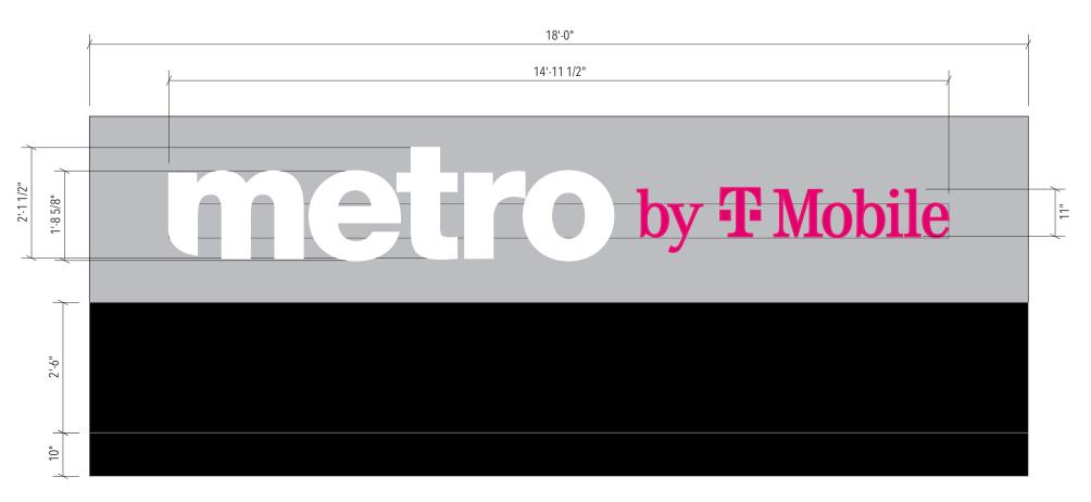
CONCEPTUAL DETAIL FACE-LIT CHANNEL LETTERS ON RACEWAY
