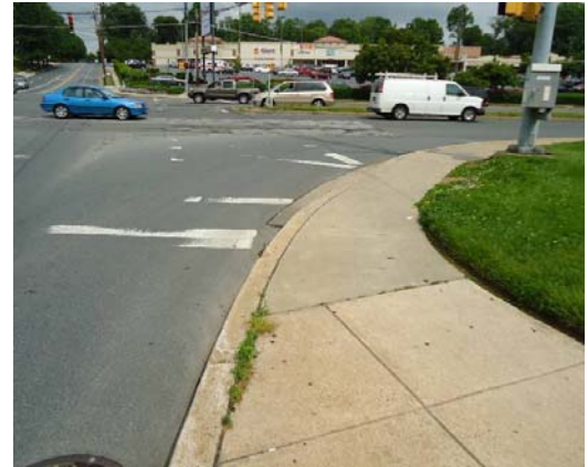
Pedestrian-vehicle conflicts were observed at a free-flow right-turn ramp (upper left and upper right). Visual limitations at a right-turn (lower left) and wide corner radii contribute to conflicts.
