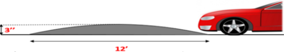
All Speed Hump are Parabolic as shown below
