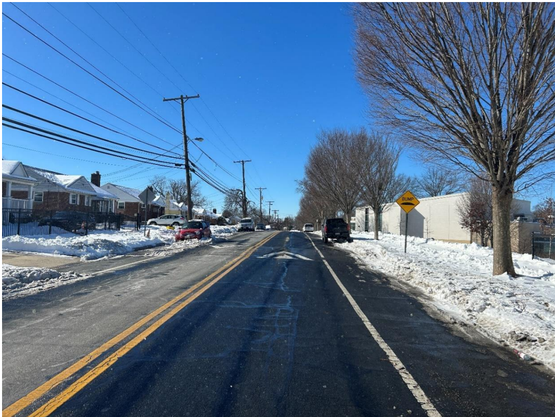
Photo 2. Limited sightline due to crest vertical curve looking west along Weller Road towards MD 185 (Connecticut Ave). Approximate crash location.
