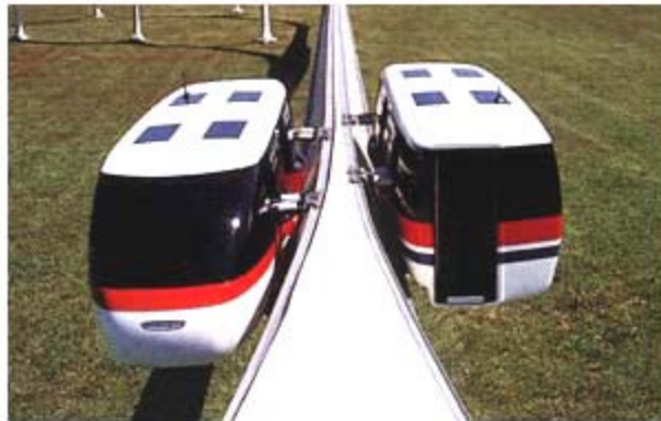
Figure 5.3. Side Straddle monorail (Futrex, 1/4 scale model, Charleston, SC)
