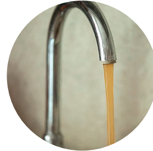
IRON rusty color, sediment, metallic taste, reddish or orange staining
