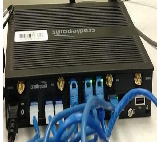
Router back with cable and power connections
