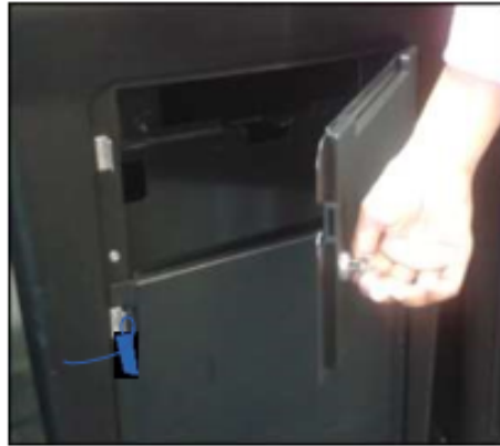
Figure 14 - Opened Emergency Ballot Compartment Door
