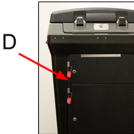
Figure 16 - New Security Seal on Emergency Ballot Compartment & Scanning Unit Opening Integrity Report
