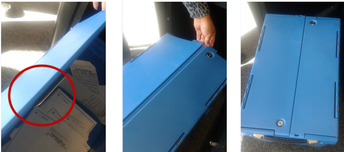
Figure 48 - "Tongue-in-groove" Fit on the Ballot Transfer Bin
