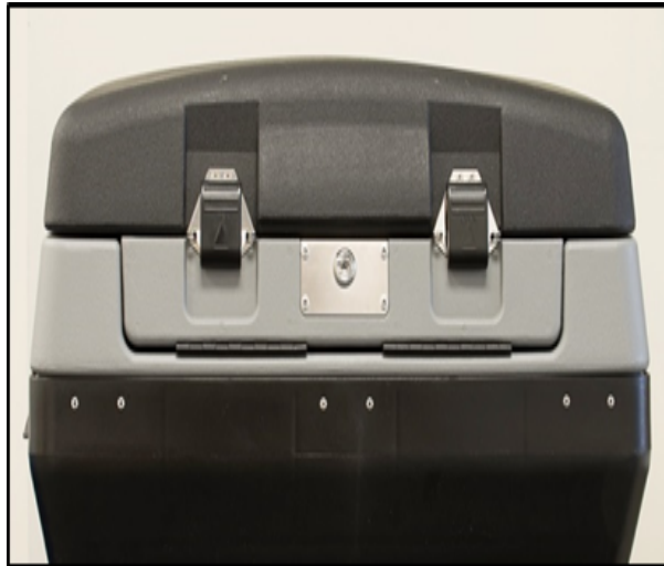
Figure 20 - Unhooked Latches on Scanning Unit
