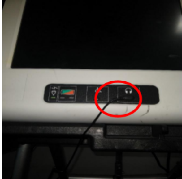
Figure 13 - Headphones Plugged in to the Audio Port of the Ballot Marking Device
