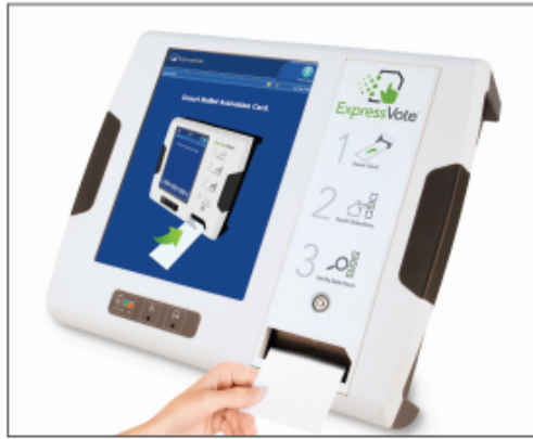
Figure 20 - Slanted Corner of the Card to the Top Right of the Ballot Marking Device
