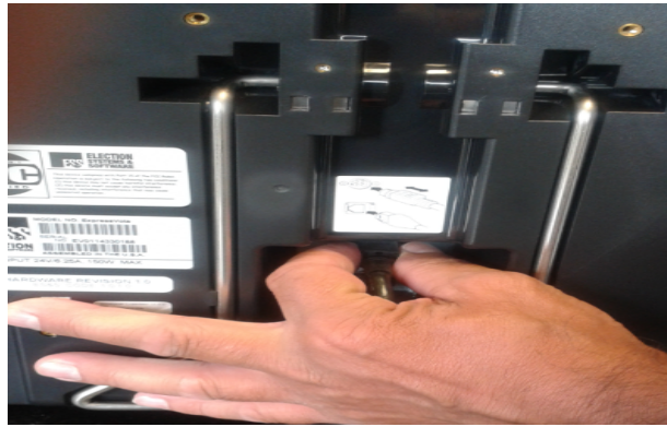
Figure 34 - Power Cord on the Back of the Ballot Marking Device
