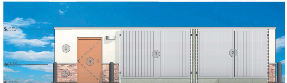
3 TRASH COMPOUND FRONT ELEVATION 3/8" = 1'-0"
