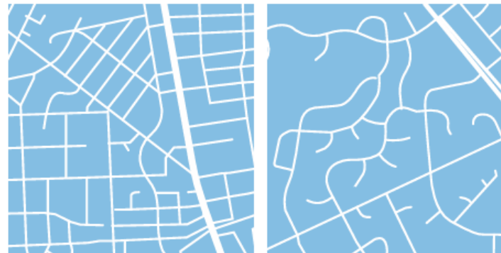
Figure 46: Higher Connectivity in a Traditional Grid of Streets (Downtown Bethesda, Left), Compared to a Conventional Cul-de-Sac Pattern of Streets (Olney, Right)
