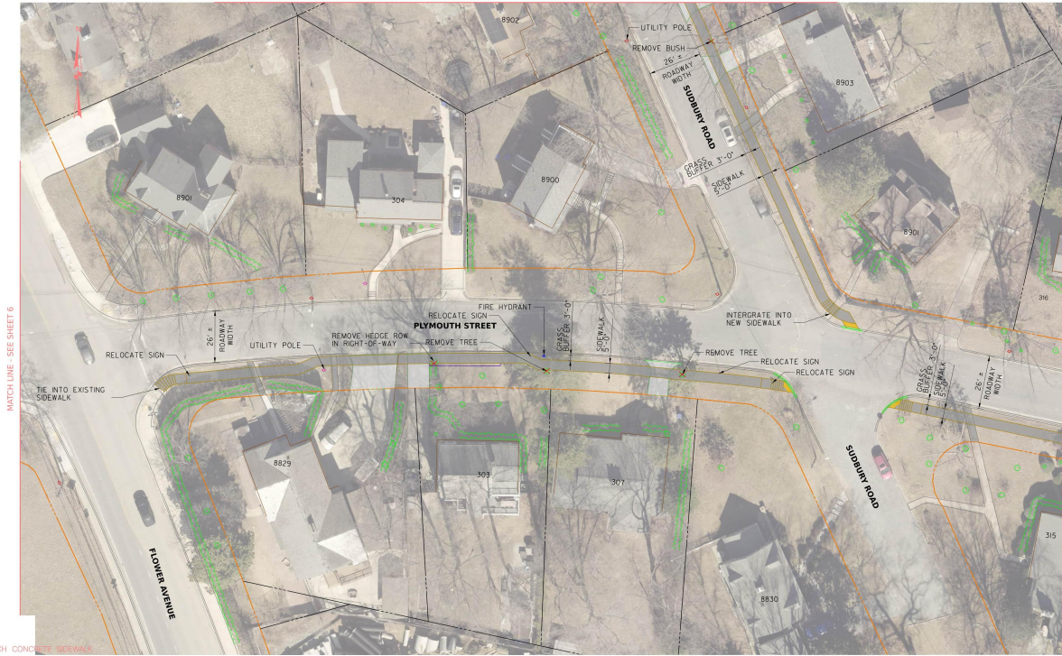
Figure 2: Aerial-based engineering plan depicting proposed sidewalk and curb improvements along Plymouth Street in Long Branch, including ADA ramps, detectable warning surfaces, driveway connections, retaining walls, utility relocations, and right-of-way limits overlaid on residential parcels.
