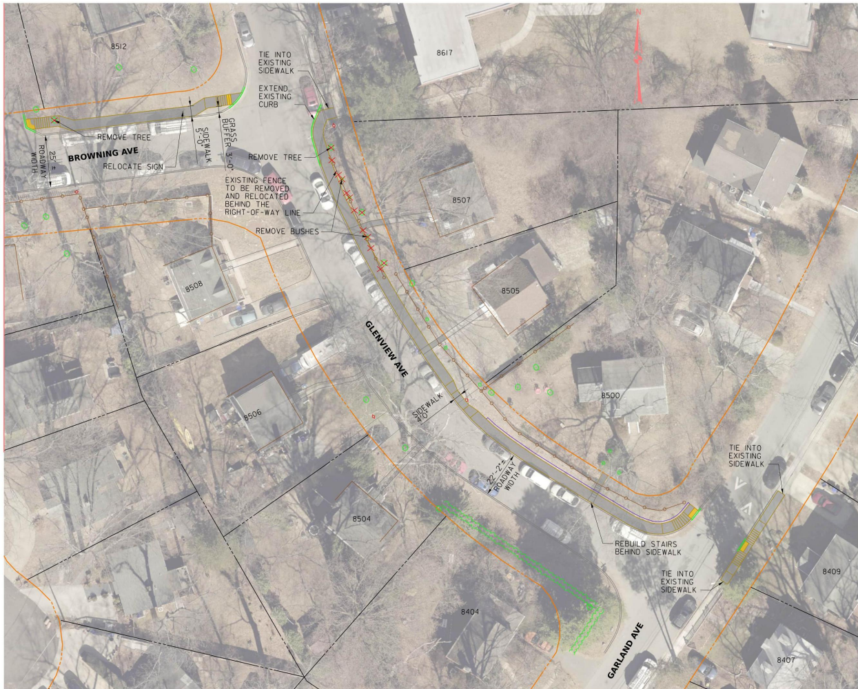
Figure 11: Aerial engineering plan of proposed sidewalk improvements along Glenview Avenue near Garland Avenue, illustrating new sidewalk segments, curb ramps with detectable warnings, driveway crossings, retaining walls, right-of-way limits, and connections to existing sidewalks adjacent to residential properties.
