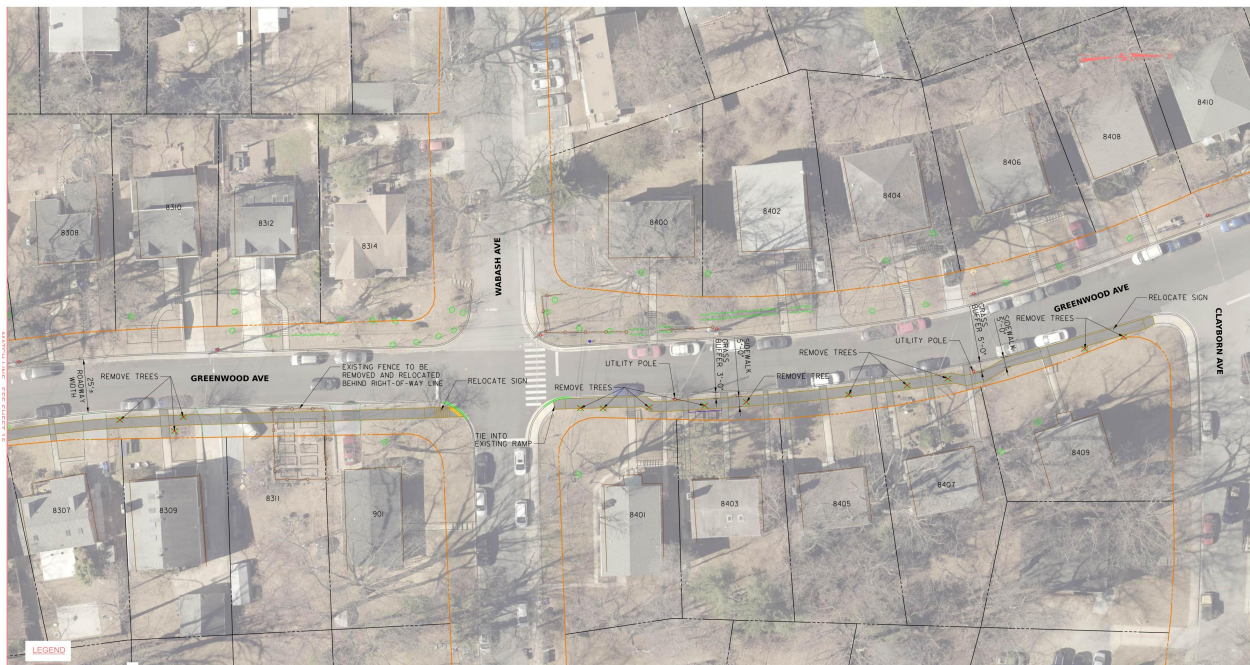
Figure 12: Plan view of Greenwood Avenue sidewalk improvements along the Long Branch Purple Line corridor, showing existing residential parcels with lot lines and building footprints, proposed ADA-compliant ramps at intersections, detectable warning surfaces at curb ramps, new curb alignments, concrete driveway replacements, retaining wall segments, approximate right-of-way boundaries, relocated signage, utility poles, and areas marked for tree removal. The drawing is overlaid on an aerial photograph and includes a graphic and numeric scale of 1" = 20'-0".
