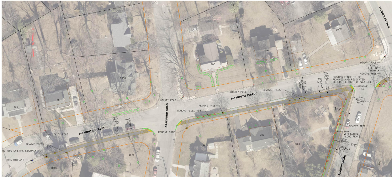
Figure 4: Aerial plan view of Plymouth Street and Bradford Road intersection showing proposed 5-inch concrete sidewalks, ADA ramps at corners, detectable warning surfaces, new curbs, tree and hedge removals, utility poles, retaining wall segments, and approximate right-of-way limits across adjacent residential parcels.
