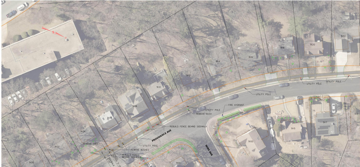
Figure 23: Aerial-based engineering plan of Long Branch Purple Line sidewalk improvements along Providence Avenue and Ware Avenue. The drawing shows property lines, house footprints, roadway edges, proposed five-inch concrete sidewalk alignment, ADA curb ramps at intersections, detectable warning surfaces, retaining wall segments, new curb locations, driveway tie-ins, approximate right-of-way limits, and utility features such as poles and a fire hydrant. Notes indicate tree and bush removal and fence reconstruction behind the proposed sidewalk. Scale graphic included (1 inch = 20 feet).
