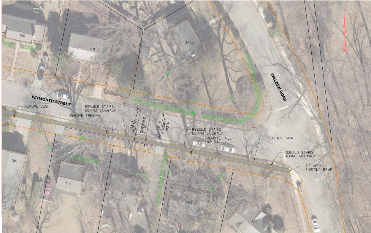
Figure 3: Aerial-based site plan of Plymouth Street and Walden Road depicting proposed sidewalk improvements, including concrete sidewalk segments, driveway connections, removal of trees and bushes, reconstructed stairs behind sidewalk, relocated sign, grass strip between curb and sidewalk, property boundaries, and adjacent residential parcels. Green dashed lines indicate vegetation or removal areas; orange lines outline project limits; annotations identify specific construction actions such as “Rebuild Stairs Behind Sidewalk,” “Remove Tree 42” Dia.,” and “Tie into Existing Ramp.”
