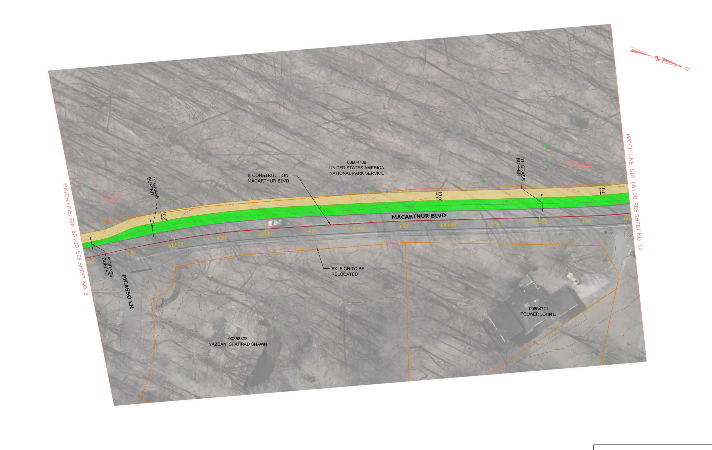
ASPHALT SHARED USE PATH GRASS BUFFER CURB AND GUTTER ---- RIGHT OF WAY PROPOSED W-BEAM GUARDRAIL ---- EXISTING CONTOUR EXISTING UTILITY POLE TREE 36" DIAMETER AND GREATER PROPOSED STORM DRAIN SCALE: 1" = 30'
