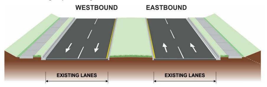
\*This typical section is for an existing four-lane section. The number of lanes in Alternative 1 would match the existing conditions.
