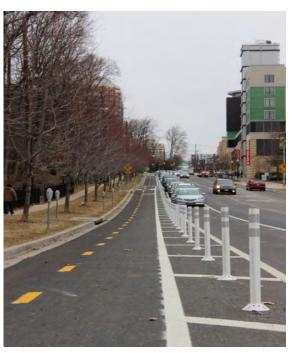
Figure 2-17: A completed two-way protected Cycle Track along Woodglen Drive in Montgomery County.
