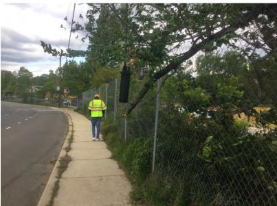
Figure 6-15 Overgrown trees and shrubs provide horizontal and vertical obstructions on the road.
