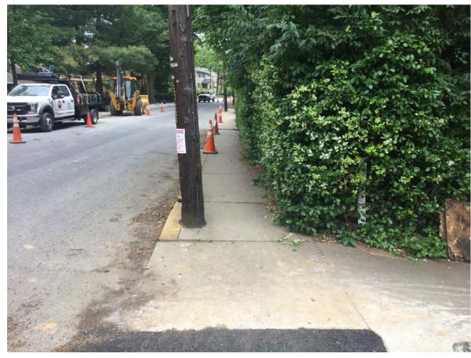
Figure 11-14 Overgrown trees and shrubs provide horizontal and vertical obstructions along sidewalks.
