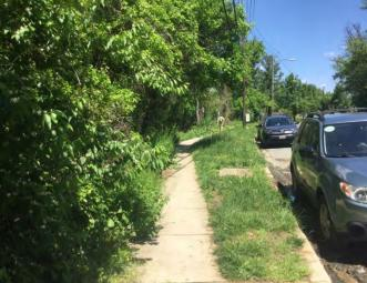
Figure 2 -20: Grass overgrowth and overgrown hedges decrease existing sidewalk width and create vertical obstructions.
