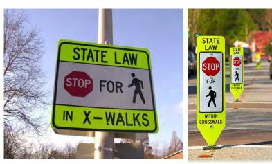
Figure 2-8 High visibility R1-6a signs are effective for uncontrolled crossings.
