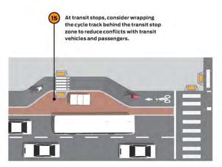
Figure 2-19NACTO suggests wrapping the cycle track behind a bus stop as one option to maintain safe access to transit.
