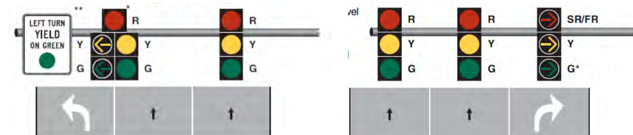
Figure 23 - Typical Positions and Arrangements of Signal Faces for Exclusive/Permissive Turn Modes. Source: MD-MUTCD
