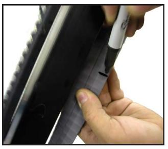
Figure 39 - Marking the Starting Point for Sanding the Belt
