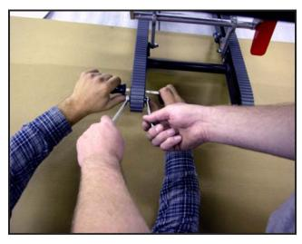
Figure 36 - Tensioning the Belt
