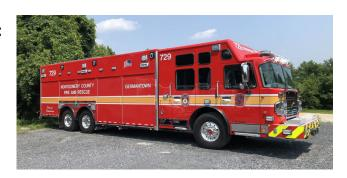
Length 42'2", Width 100" Cab (9'8" mirror to mirror), Height 11'2", Gross Vehicle Weight 77,000 lbs
