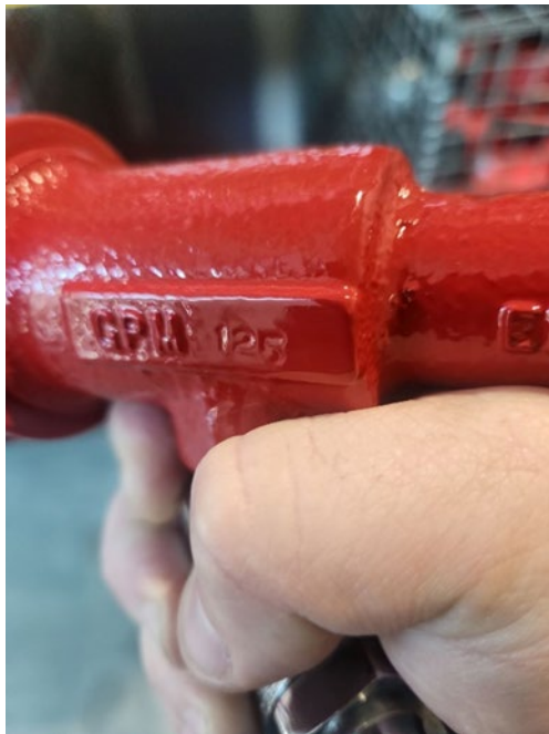
Figure 3 - 125 gpm eductor; note stamp with gpm rating. This must match the nozzle.
