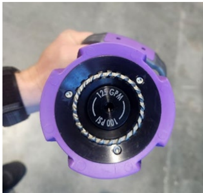
Figure 1 Elkhart Nozzle with purple bumper. Note gpm rating on insert.
