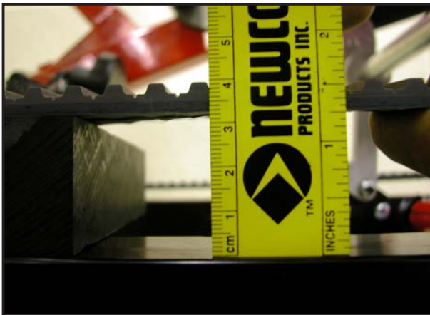
Figure 37 - Checking Tension with Chair Laying on Its Tracks on a Work Bench
