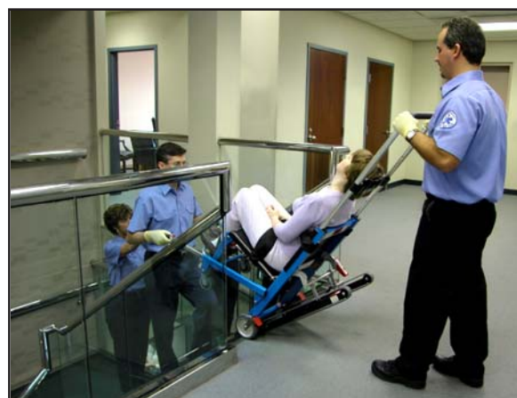
Figure 24 - Track Belts Engaging Top Step
