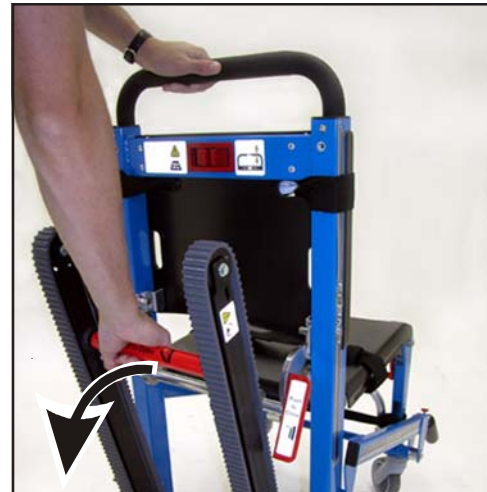
Figure 12 - Opening the Track
