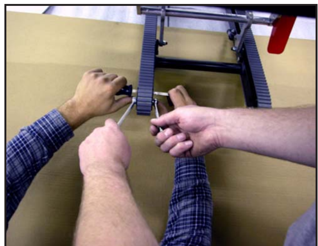
Figure 36 - Tensioning the Belt
