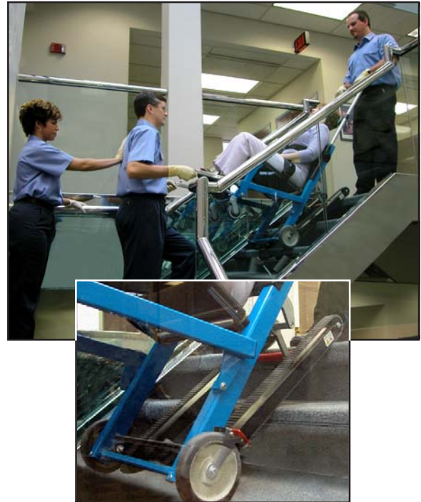
Figure 25 - Establishing the Glide Angle
