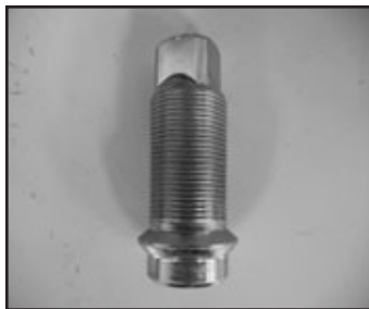
Inner Cap Nut Note: The top of the inner cap nut will have thread direction identified on the end of the nut.
