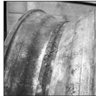
Discoloration of Wheel
