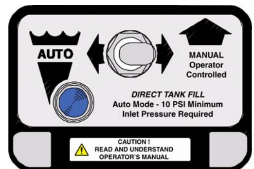
Figure 2-3: AutoFill Control Panel AUTO / MANUAL
