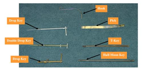
Insert the appropriate key through the hole on the front of the car door until the tip drops.
