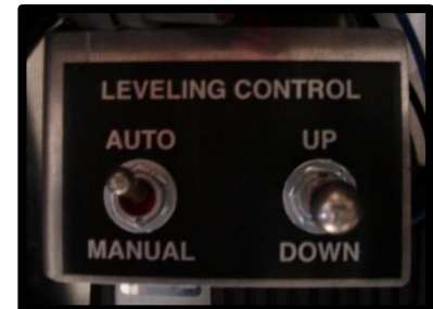
Platform Leveling Controls
