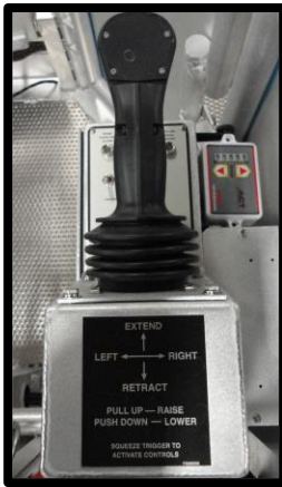
Aerial Joystick from top looking down over control panel
