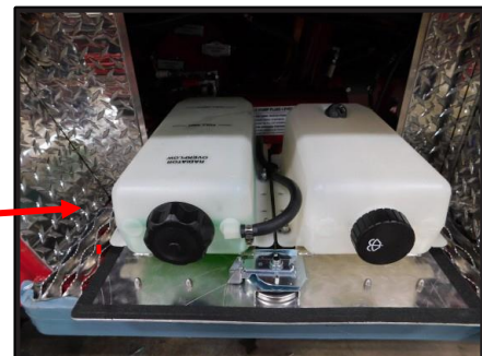
Fluid reservoirs for Washer Fluid (R) and Radiator Overflow (L)
