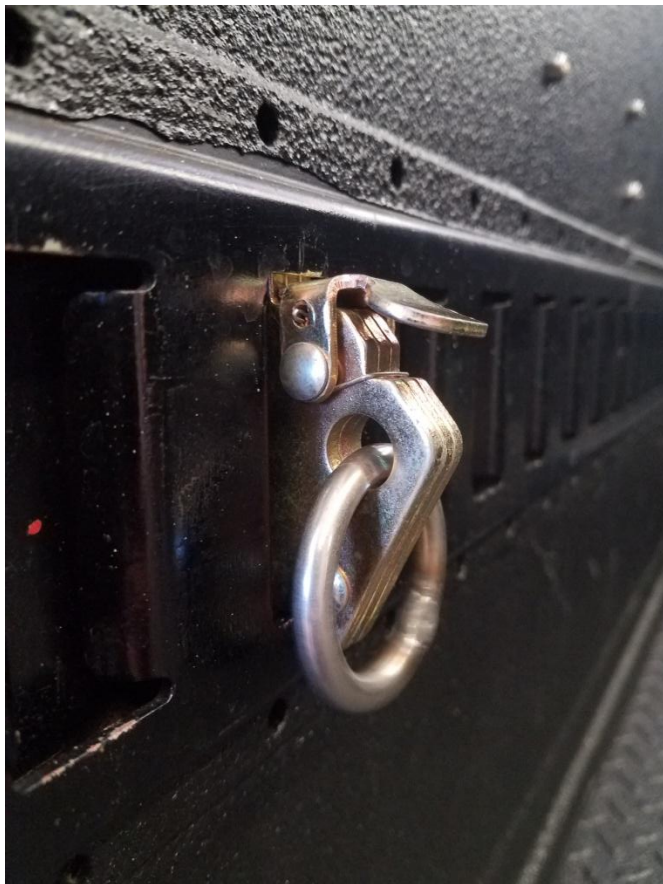
E-trac brackets and ratchet straps utilized to secure stokes basket for patient evacuation.
