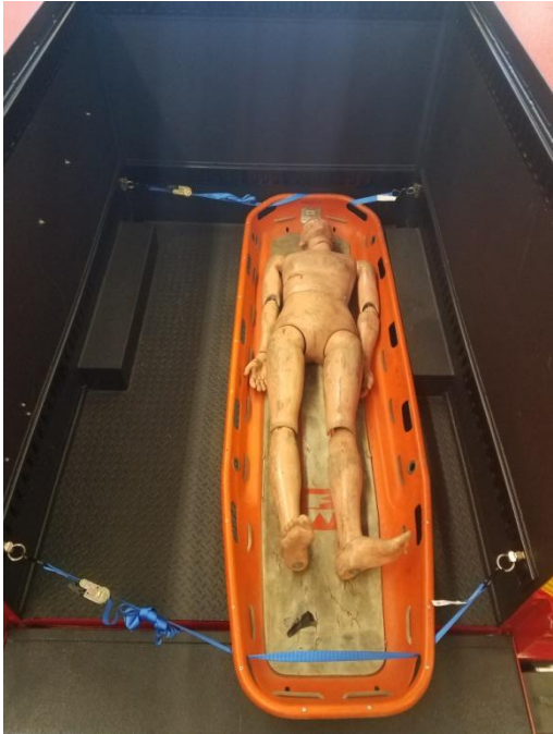
E-trac brackets and ratchet straps utilized to secure stokes basket for patient evacuation.
