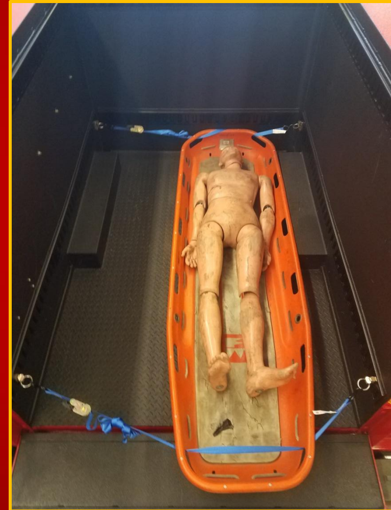
E-trac brackets and ratchet straps utilized to secure stokes basket for patient evacuation.
