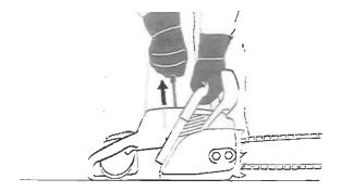
3. Kickback is a sudden rearward motion of the saw that occurs when the upper tip of the bar touches an object. The chain can come in contact with the operator and cause serious injury.
