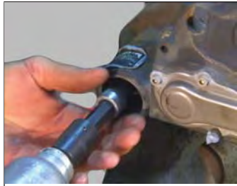
FIGURE 67 - REMOVE THE CALIPER BOLTS
