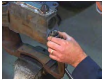
FIGURE 78 - POSITION THE NEW BUSHING
