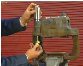
FIGURE 70 - INSTALL THE REMOVAL TOOL
