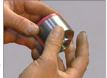
FIGURE 82 - POSITION THE NEW BOOT IN THE INSTALLATION TOOL (T7)
