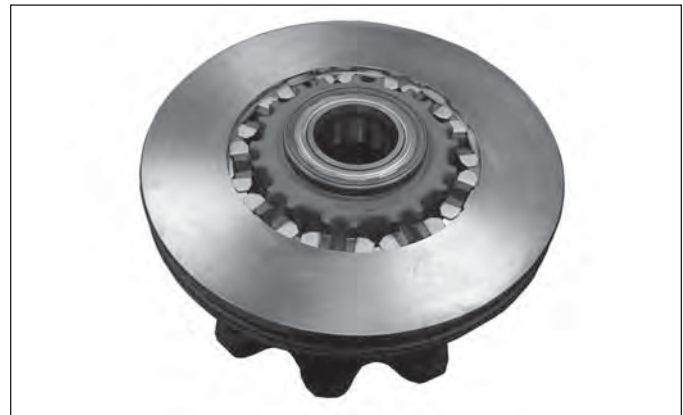
FIGURE 90 - INTERMEDIATE ELEMENTS (SPACERS) INSTALLED
