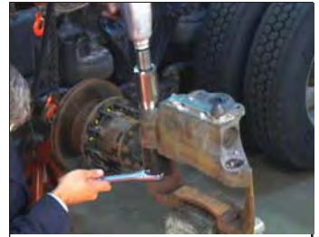
FIGURE 71 - REMOVE THE LONG GUIDE PIN
