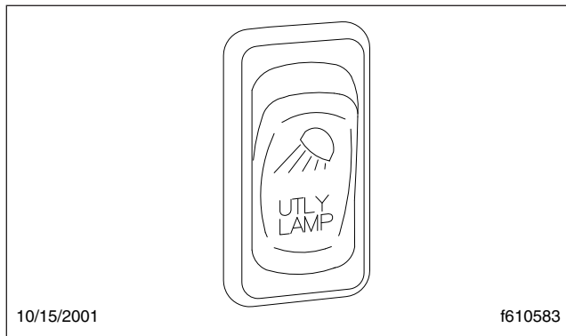
Fig. 4.7, Utility Light Switch
