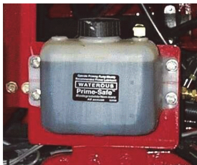
Figure 4-2: Primer Pump Lubrication Fluid or Oil Reservoir
