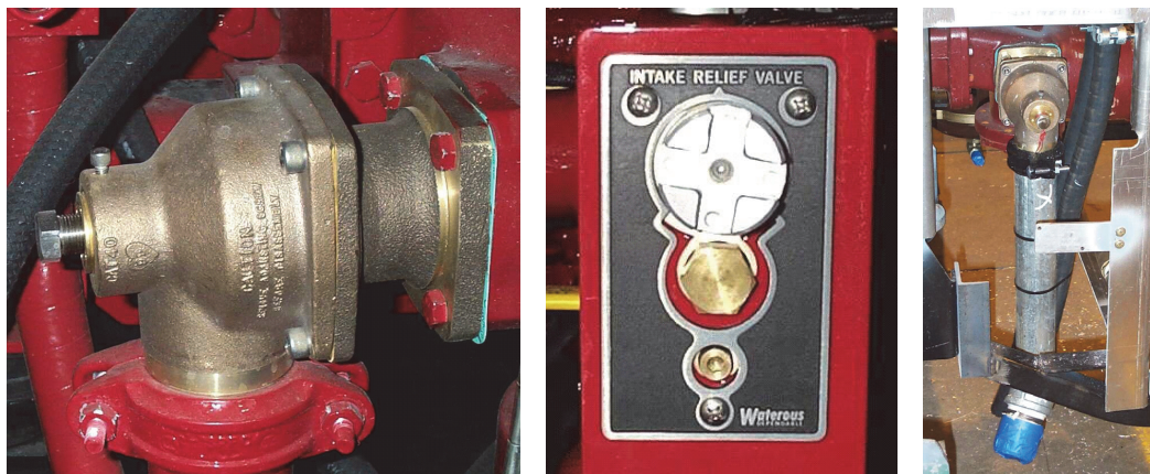
Figure 2-1: Typical Intake Relief Valve ( relief outlet pipe with threaded end shown on right )
